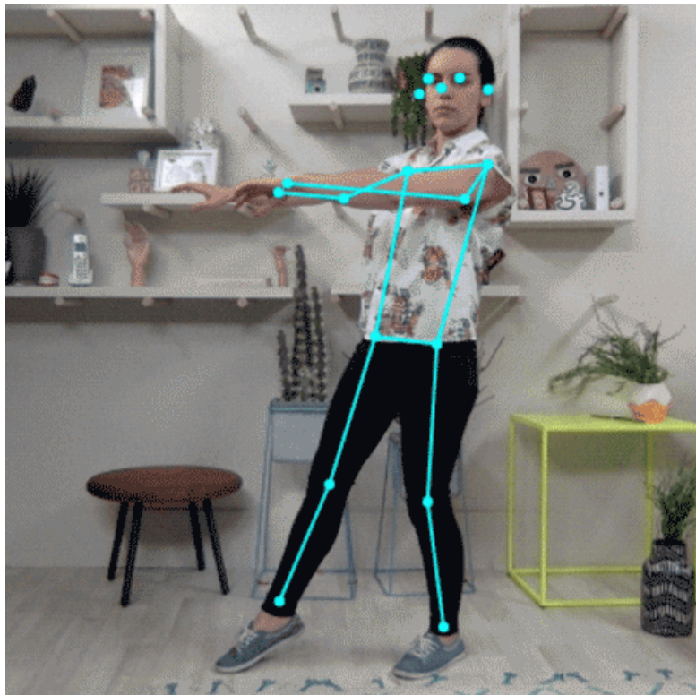
Figure 12. Detecting human posing via the PoseNet browser framework [30]
